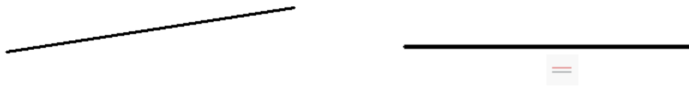
Left: Line drawn at an arbitrary angle; right: Line snapped flat by horizontal constraint
