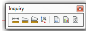
From left to right: Distance, Area, Mass Properties, ID Coordinates | List Entity Data, Drawing Status, Time Variables
