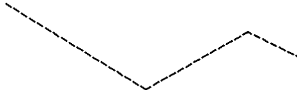
Drawing line segments with hidden linetype automatically applied
