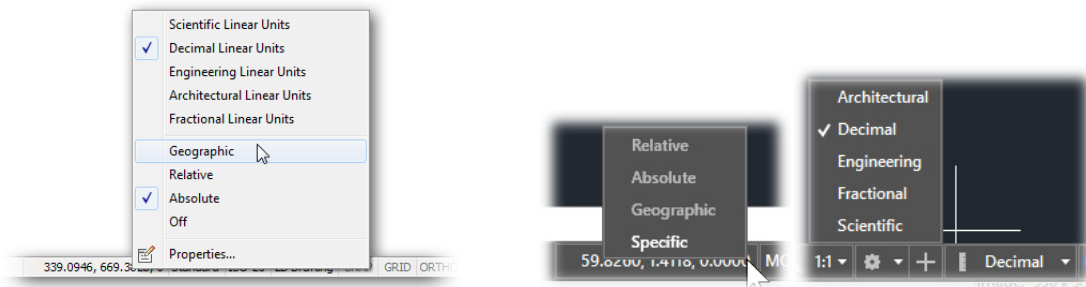
Left: Accessing units formats from the status bar in BricsCAD; right: AutoCAD requiring two status bar buttons
